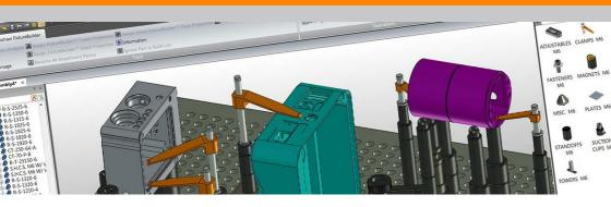
FixtureBuilder is a 3D software package designed to allow the creation and documentation of metrology fixturing set-ups. It can also be used to assist with offline programming.
